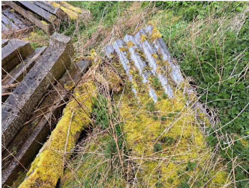
Image 8.16 Fly-tipped material - suspected Asbestos CM
