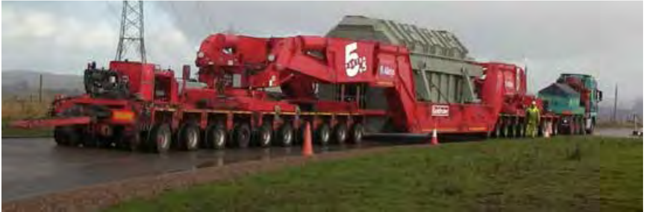
Figure 2 Example Transformer Load Transporter
