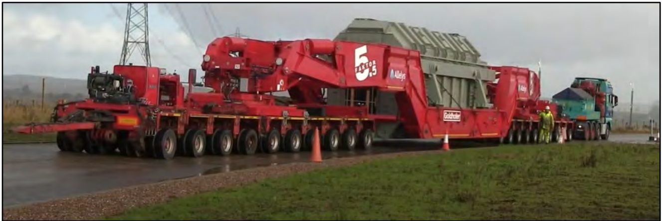
Figure 6 Example Transformer Load Transporter
