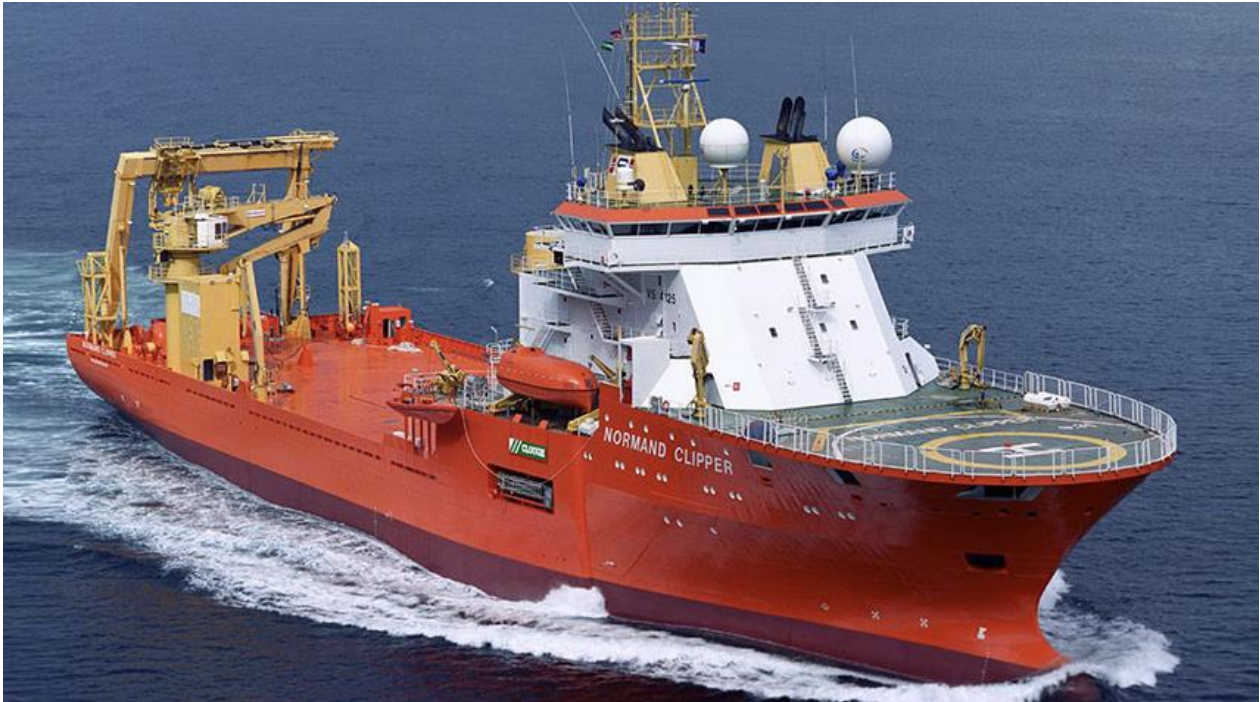
Figure 5.16 A Normand Clipper Cable Lay vessel involved in IAC cable installation at the Kincardine windfarm.
