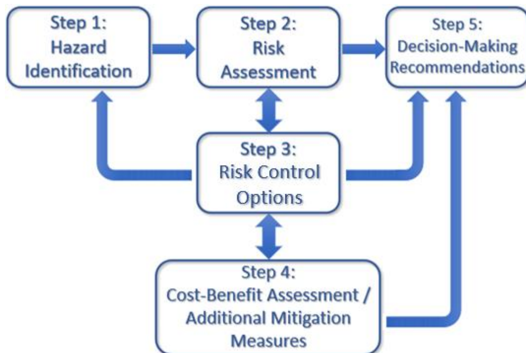
Figure 3.1: Flow Chart of FSA Methodology
